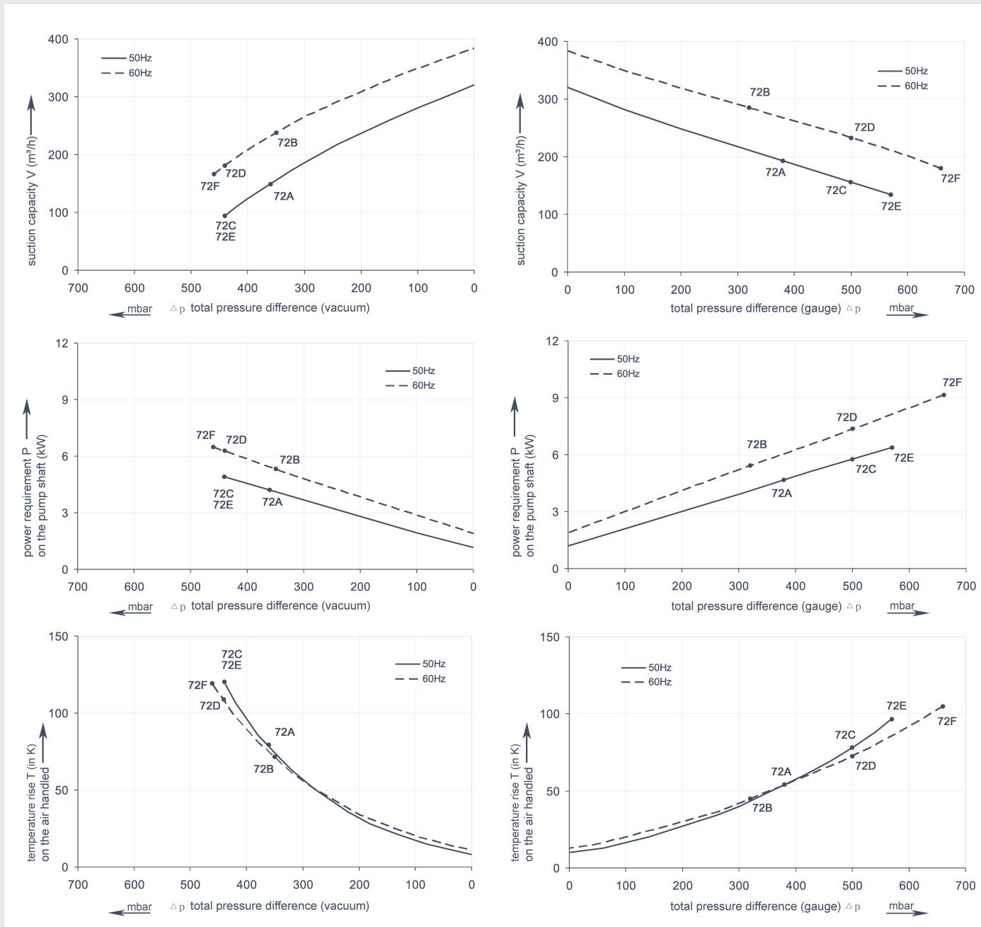
The performance curves are based on air at a temperature of 15 °C and an atmospheric pressure of 1013 mbar with a tolerance of +/- 10 %. The total pressure differences are valid for suction and ambient temperatures up to 25 °C.
