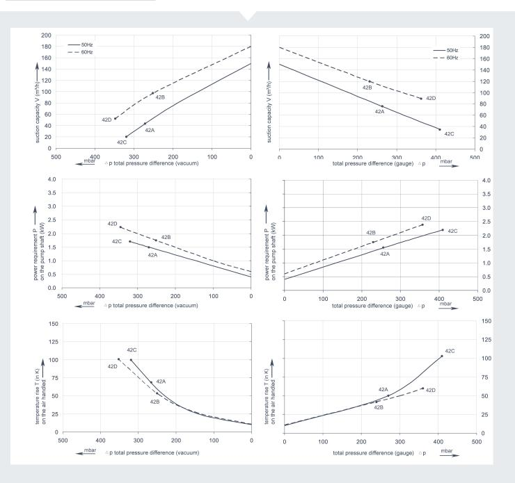
The performance curves are based on air at a temperature of 15 °C and an atmospheric pressure of 1013 mbar with a tolerance of +/- 10 %. The total pressure differences are valid for suction and ambient temperatures up to 25 °C. For other conditions please confer with us.
