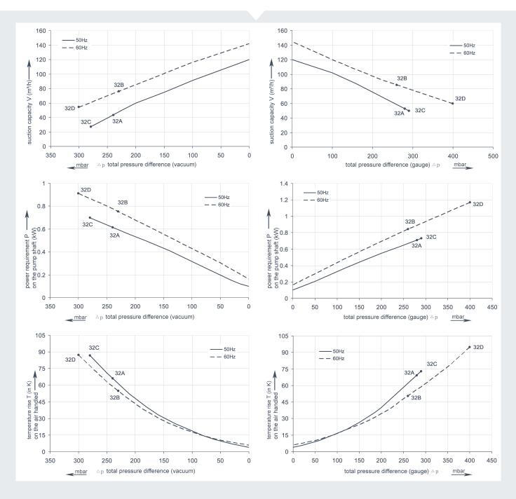
The performance curves are based on air at a temperature of  $15\,^{\circ}\text{C}$  and an atmospheric pressure of  $1013\,^{\circ}\text{mbar}$  with a tolerance of  $+/-10\,^{\circ}$ . The total pressure differences are valid for suction and ambient temperatures up to  $25\,^{\circ}\text{C}$ . For other conditions please confer with us.
